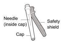
• Injection Needle with safety shield. You may use a 25, 26 or 27 gauge needle.
